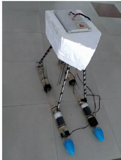
图 10 半潜式无人艇的实物模型 Fig. 10 Physical model of unmanned semi-submersible vehicle
